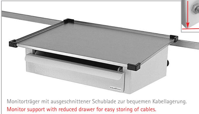
The monitor support is mounted with two rail clamps on wall rails. Two variable rods support the unit against the wall. The version bridges a distance of 80 mm from the front end of the wall rail to the wall.
